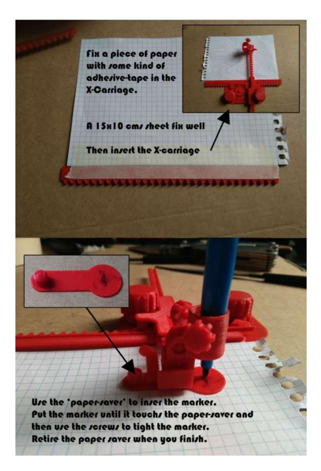
The screws: Put a marker pen and adjust the screws
