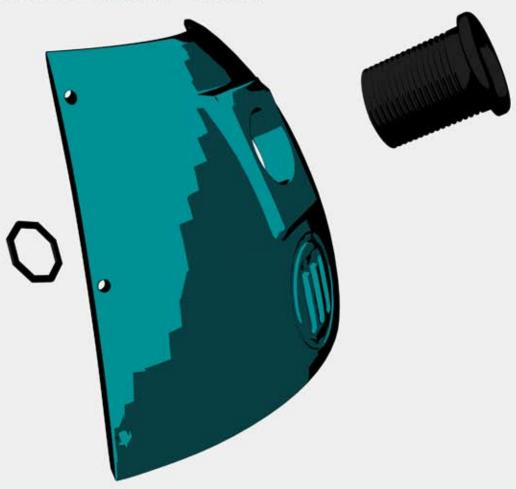
9.) Connect side.stl to face.stl using M3 x 40mm (be sure to use 40mm, since later on, we will see a reason for the extra length) and legBracket.stl. Be sure to place the tapered end of legBracket.stl facing up (as shown).
