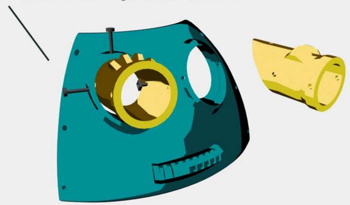
3.) Attach leftJet.stl to side.stl using 3 x M3x16mm screws/nuts
