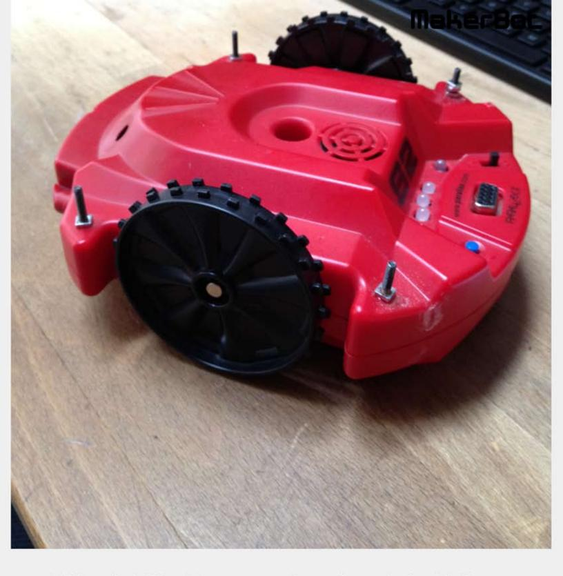
22.)Attach 4 M3 x 30mm screws/nuts through the 4 holes that you just drilled, as pictured.
