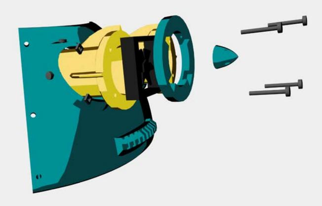
7.) Attach arcade button through hole in side.stl (some sanding might be required to widen holeif slight shrinkage occurred). Attach plastic nut that was supplied with the button.
