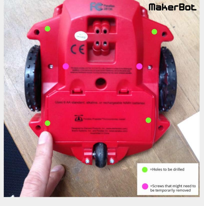
21.) Using a small phillips screwdriver remove the 4 corner screws. You might also need to temporarily remove the 2 closest to the wheels in order to "spread and rattle' the initial 4 corner screws loose, they sometimes stick. Just replace the 2 near the wheels when the corner screws are out, to keep the body together while we... 22.) Drill all the way through the 4 corner holes using a bit that is roughly the size of an M3 screw ( or a bit larger).
