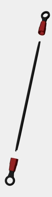
19.) Using a crimping tool, attach your electrical 'loop' couplers to both ends of your 35mm lengths of 100lb picure hanging cable. I also put a drop of cyanoacrylate glue in each coupler beforehand, just to be safe. Make 4 of these.
