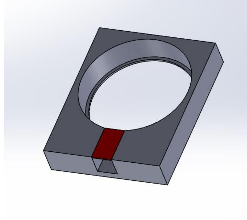
By default, the base and charger cap print with a thin connector (shown in red) to help reduce warping. Cut these prior to assembly.
