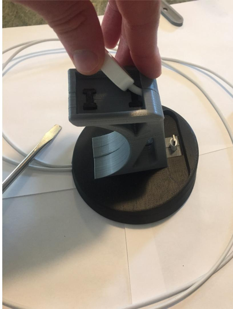
Press the two clips into the pockets under the watch charger. It helps to use a flathead screwdriver.
