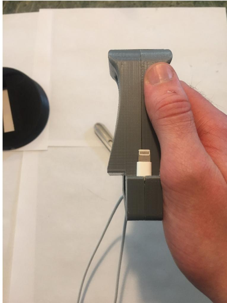
To disassemble: Remove the base, then grab one half and firmly pull down the other half while rocking it back and forth.
