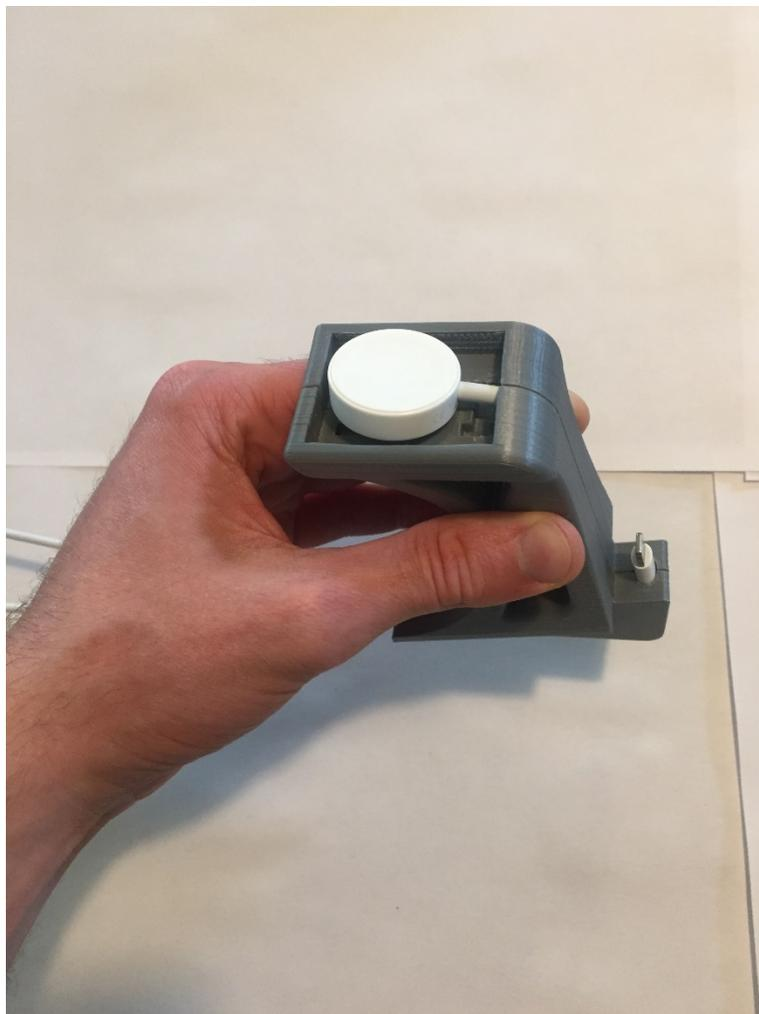
Bring the two halves together, and remove the charger cap from the watch charger.
